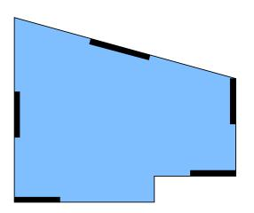
Vertical lateral force-resisting elements not parallel to or symmetric about the major orthogonal (x, y) axes.
