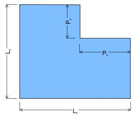
Largest notch on diaphragm P<sub>y</sub>>0.15L<sub>y</sub> AND P<sub>x</sub>>0.15L<sub>x</sub>
