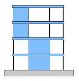
In-plane offset of lateral force-resisting elements resulting in overturning loads being supported by a different element (i.e. column, transfer beam) below.
