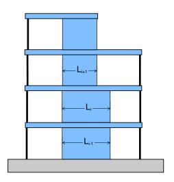
Checking each level, horizontal dimension of the seismic force–resisting system >130% of adjacent story.
