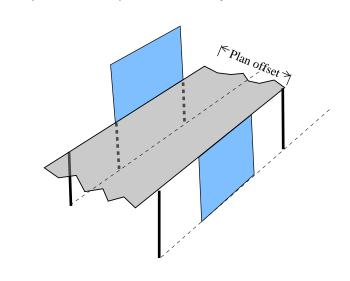
Horizontal discontinuities in a lateral force-resistance path by offsets of the vertical elements perpendicular to the axis of the vertical element.
